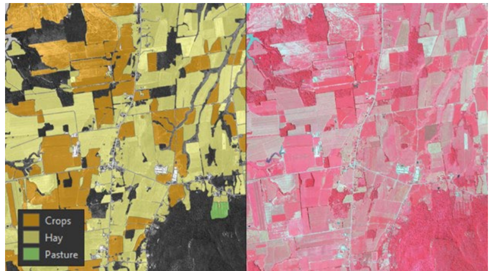
Figure 28 (Top): Lidar-derived elevation data is used to help create high-resolution land cover data which in turn is used to help analyze the impacts of agricultural and other land uses on Vermont waterbodies. Source: Colin Dowey/ANR
