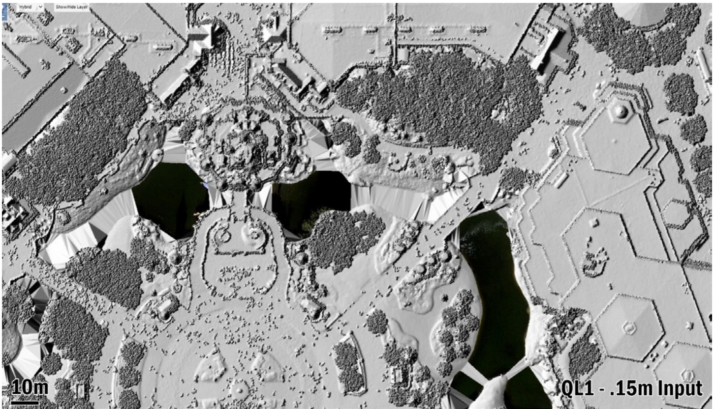
Figure 20 (Top): Hillshade derived from .35m DEM input, simulating QL1 source data. Data Source: USGS/opentopography.org
