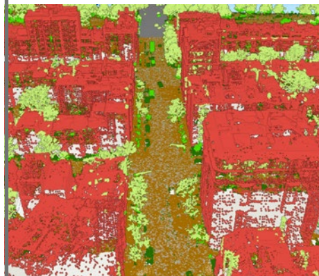
Figure 12 (Left): QL2/2pts/sq.m point cloud colored by classification. Brown points are ground, grey are unclassified.
