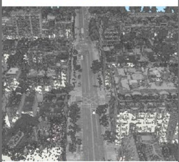
"QL1" Capture ~8 points per sq. meter Proposed VT Lidar-derived Elevation Resolution
